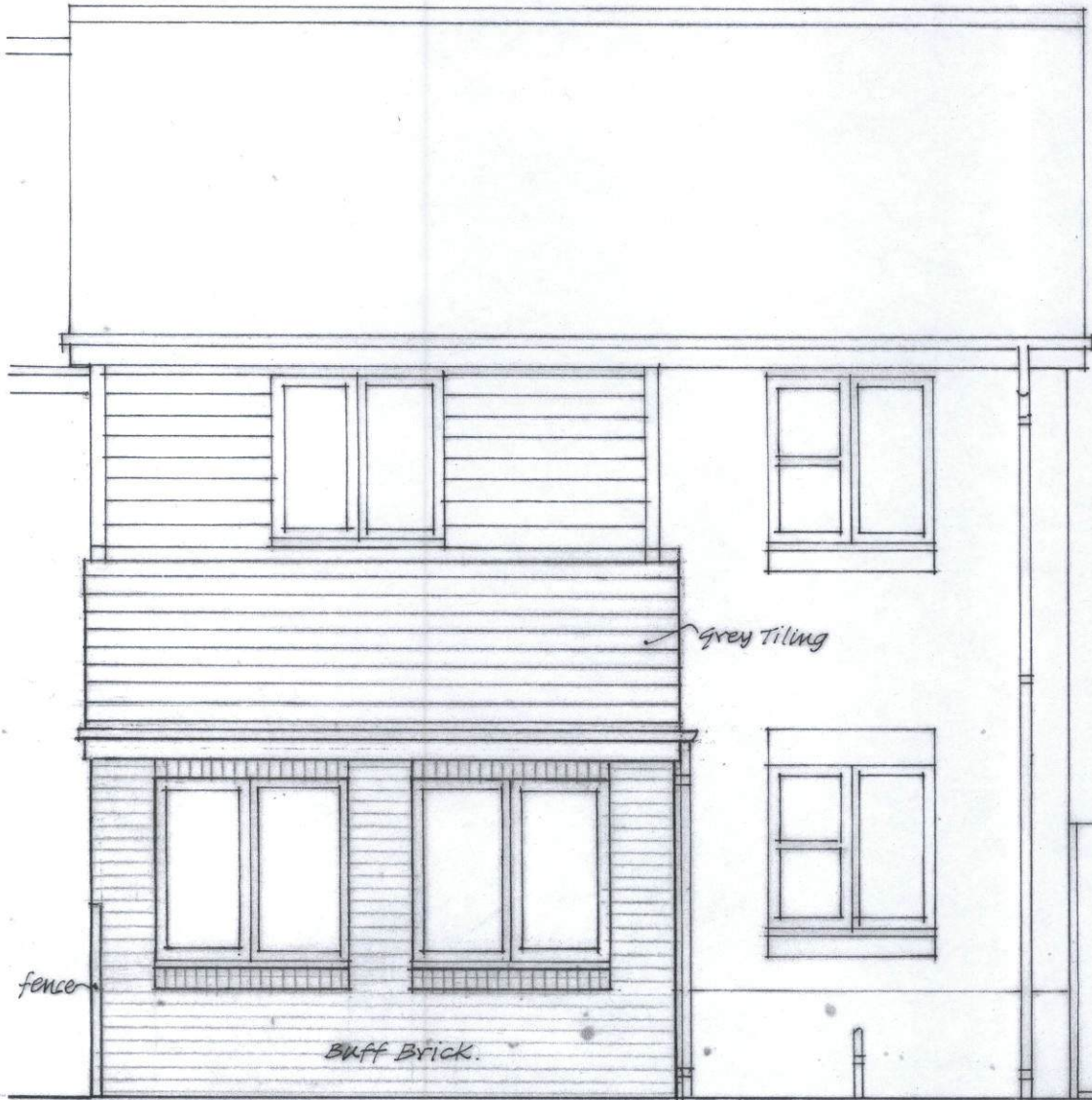
Proposed Rear Elevation 1:50
